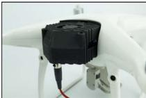
**Step 8:** Insert the Power Key to power up the aircraft. The aircraft will initialize. It is recommended to operated with the lid closed to prevent possible entry of foreign matter.
