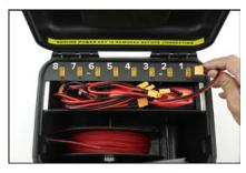
**Step 3:** Check the voltage meter regularly. Full charged is 25.2V. Once the system is below 20V, the low voltage beeper will sound off. You should land the craft immediately.
