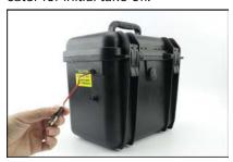
**Step 5:** For the Mavic 2, connect the tether cable to the Air Module as shown. Insert the cable snuggly into the slot located on the side wall.
